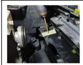
Mark out where the end brackets need to be drilled and drill a 6mm hole.
