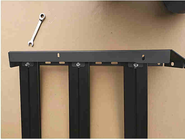
2 fix slats on one side support with hex bolts M8x15
