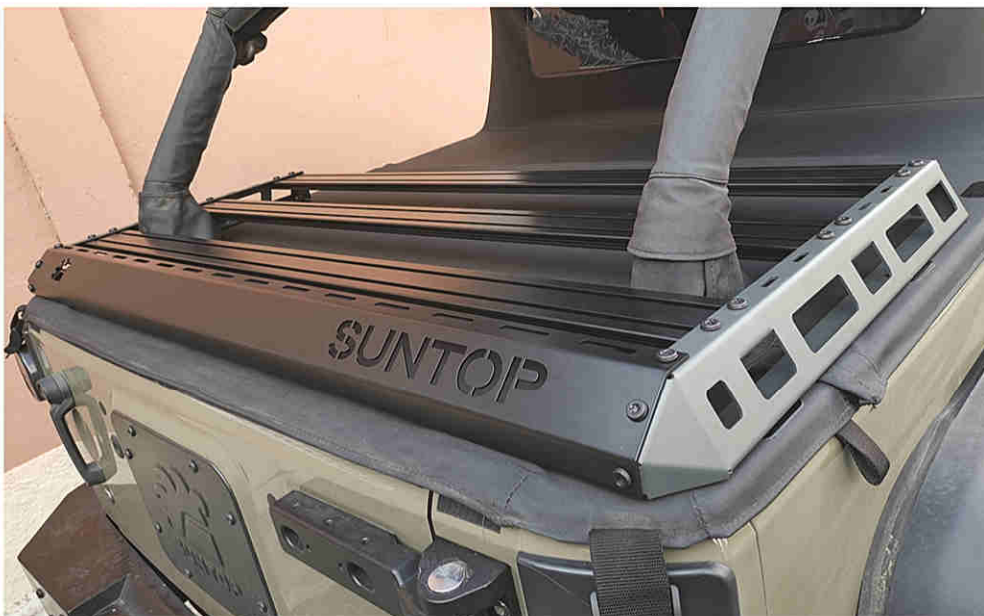
10 fix side supports with torx bolts and threaded inserts. DO NOT TIGHTEN
