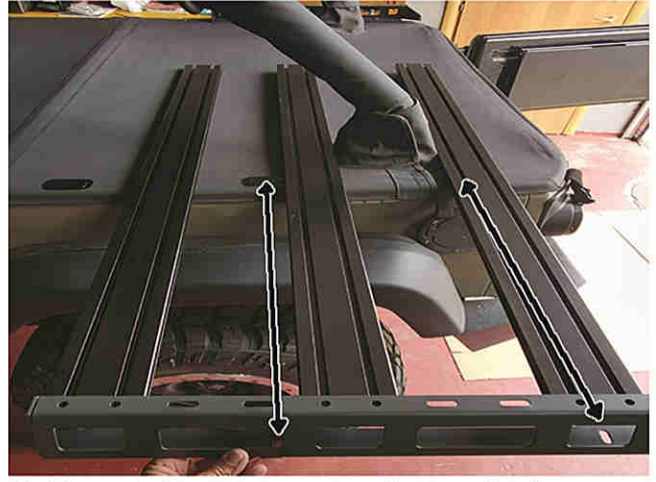
3 Check the correspondance between side supports and threaded holes on the car
